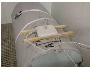
LIFERAFT STORED FOR 50HRS AT -70^{\circ}\text{C}
